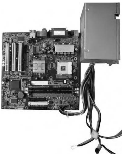
Figure 4.8 Power supply connected to motherboard.
