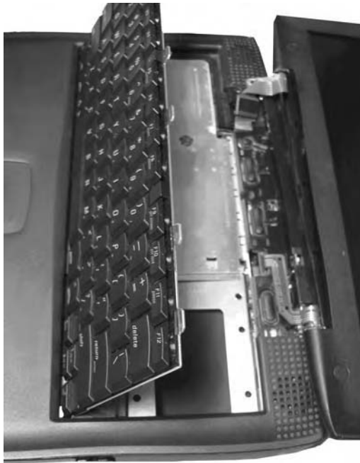
Figure 4.15b Lifting keyboard to access laptop components.
