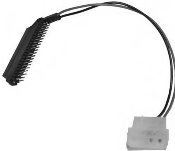
Figure 9.1 Laptop to IDE hard drive adaptor.
