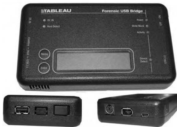
Figure 9.4 Tableau forensic USB bridge right blocker.
